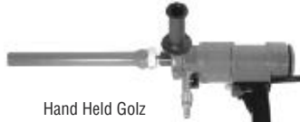
Hand Held Golz 9 amp / 120 vac Weight: 14 lbs. 650 / 1300 rpm 4" Capacity 1", 1 1/2", 2", 2 1/2", 3", 4" Diamond Core Bits Water Required
