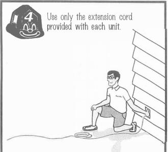
Plug each blower into a 110 volt electrical outlet. Make sure the outlet has either a dedicated 20 AMP or larger circuit, or a 30 AMP fused circuit. The blower should be the only thing plugged into that circuit. If two blowers are required they must be on separate circuits.
