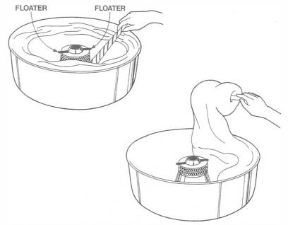
When stopping operation for the day or any prolonged period, it is a good idea to run all of the sugar out of the floss head. When empty, turn heat to the highest setting for approximately one minute to remove carbon from ribbons. NEVER ALLOW WATER TO ENTER THE FLOSS HEAD. A damp cloth will be sufficient to wipe off floss head after use, BUT BE SURE TO UNPLUG MAIN ELECTRICAL SUPPLY CORD FIRST. Make sure all parts are dry before resuming operation.
