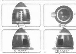
B Indicates Pre-Installed Blower Tube locations.
