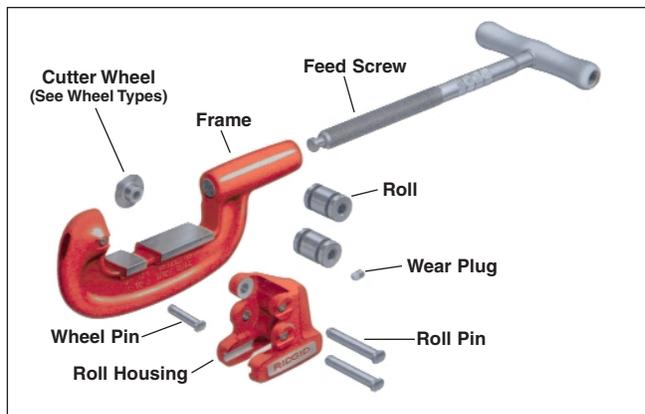
Single wheel cutters must be rotated through 360° to complete the cut. Should there not be enough space to do this, a four wheel cutter should be used. By swinging the cutter through an arc of 120° each wheel will track to the groove cut by another wheel and thus completes the cut.
