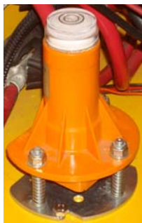
Figure 4-11. Level Sensor Pendulum Based
