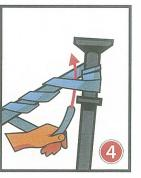
4. Insert end of webbing through the opening hole as shown above.
