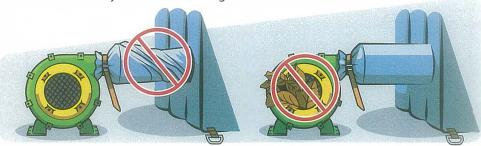
1. Close all unused inflation tubes. 2. If your inflatable includes a deflation zipper, ensure that it is closed and sealed with the velcro flap.
