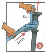
5. As you pull the webbing to tighten, push knot toward stake to lock in place.
