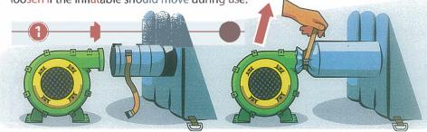
• Be sure to straighten any kinked inflation tubes. Make sure the blower air intake is clear of leaves or any other debris during use.
